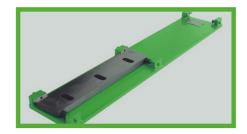
The adjustment of all knives takes place outside the cutter-mill in a setting gauge, which is included in the scope of delivery. This eliminates tedious adjustment work inside the machine.
