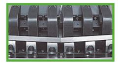
The rotor and its knives can be adjusted for various tasks. The rotor is designed according to contemporary v-cut layout guaranteeing a consistently high grinding quality.
