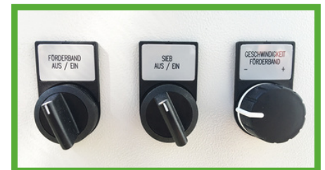
High-quality control incl. frequency converter
