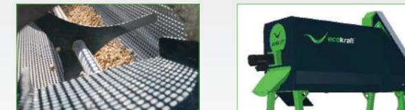
Dust-free pellets represent a high quality standard. Thanks to the innovative sieving plant from **ECOKRAFT**, the pellets are initially transported away gently using a conveyor and are thus cooled in a natural manner. During sieving, the pellet breakages (dust and pellets that are too short) are sorted out. This process represents a significant value increase for pellets for resale.
