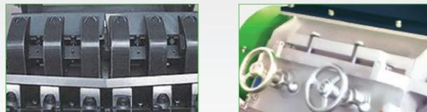
The **ECOKRAFT cutter-mills** are perfectly suited to fray the structure of already small and light biomass and some plastics. The materials are shred to a size that allows pelletization (6-8mm) and can be fed into the pellet-mills. The robust design, accessibility of vital areas and its strong construction paired with the relatively small power consumption make this cutter-mill ideal for an cost-effective and efficient pre-treatment of your source materials.
