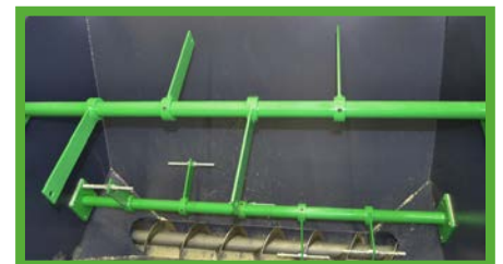
Integrated agitator to prevent bridging with very light material
