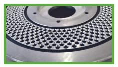
High quality hardened flat dies for different pellet diameters and different press channel lengths available.
