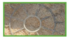
The mixer located in the material hopper prevents possible "bridging" of very light materials. Furthermore, strong magnets are integrated on the mixer, which can sort out possible foreign bodies such as nails or metal chips.
