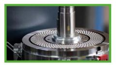
High quality hardened flat dies available for different pellet diameters and different press channel lengths.
