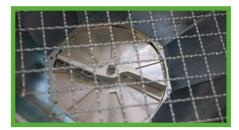
The mixer located in the material hopper prevents possible "bridging" of very light materials. Furthermore, strong magnets are integrated on the mixer, which can sort out possible foreign bodies such as nails or metal chips for the most part.
