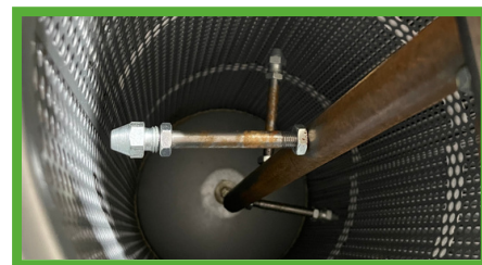
Cleanable long life filter cartridge for low wear costs
